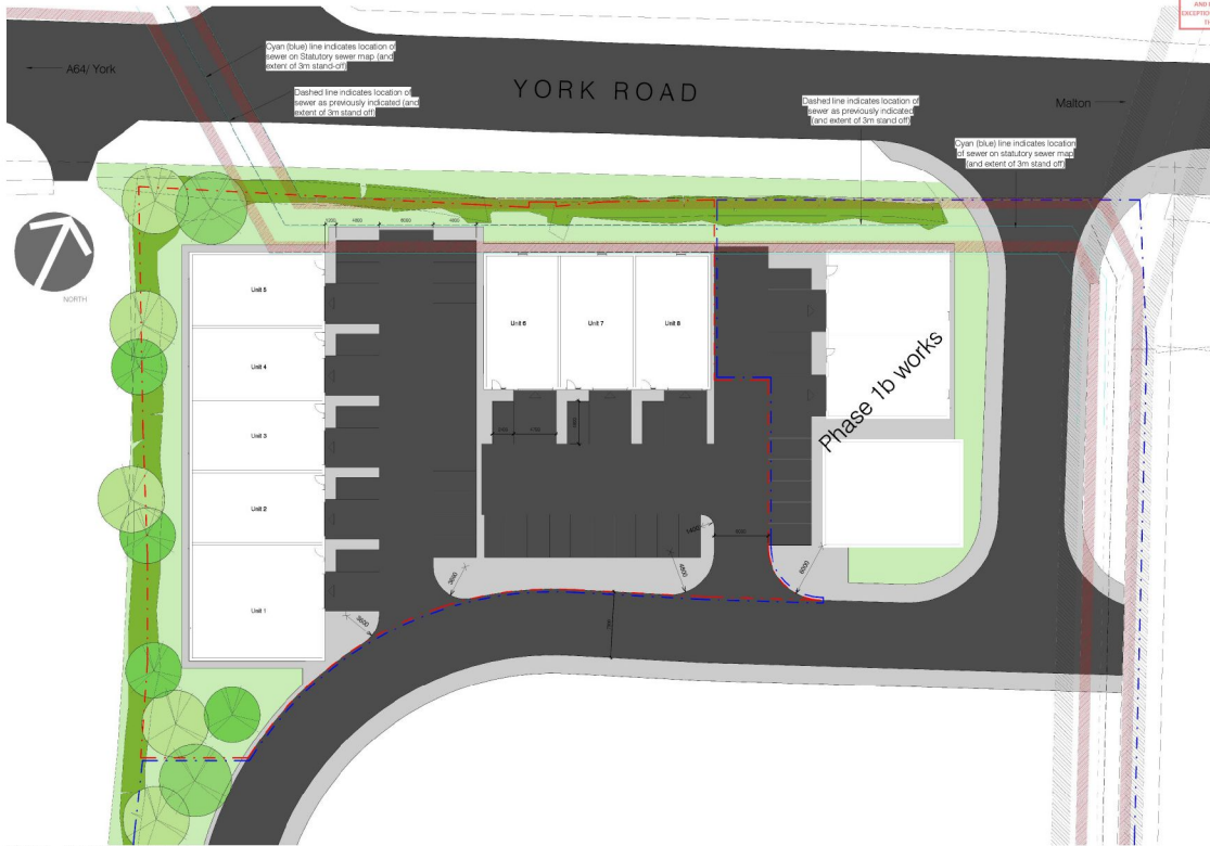
Site Plan - Location of existing Sewer 1:200
